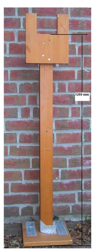
**Important:** This brace must be secured against fall over with two ropes from the mast to the cleats at the stern.
