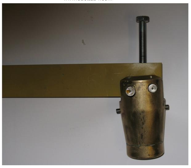
Subtract the body from the propeller shaft with the screw (M12)
